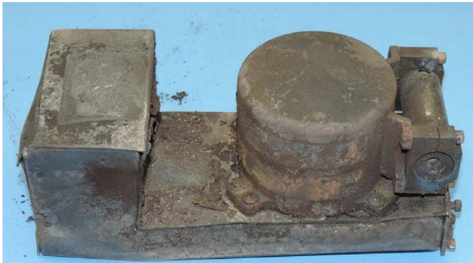
Figure 2. CVR in NTSB laboratory.
