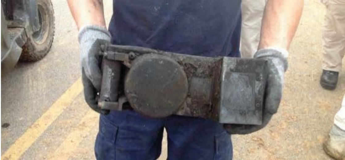
Figure 1. CVR after removal from aircraft.
