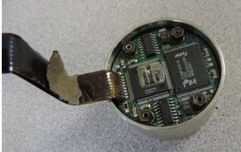
Figure 5. Stacked memory boards within memory puck.
