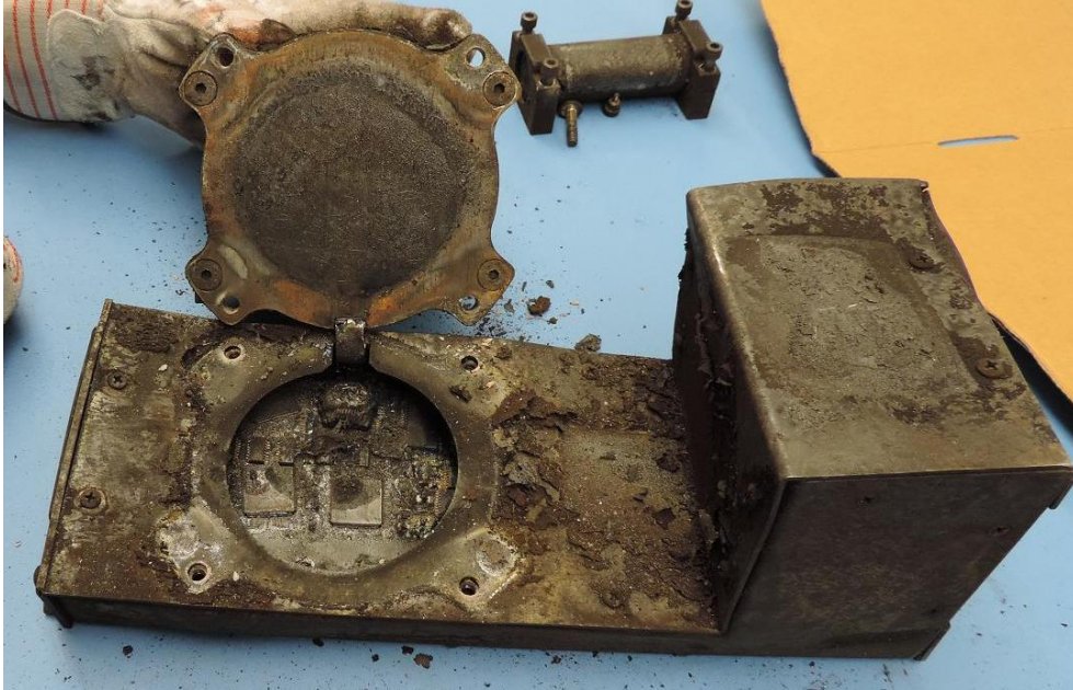
Figure 3. Removal of CSMU.
