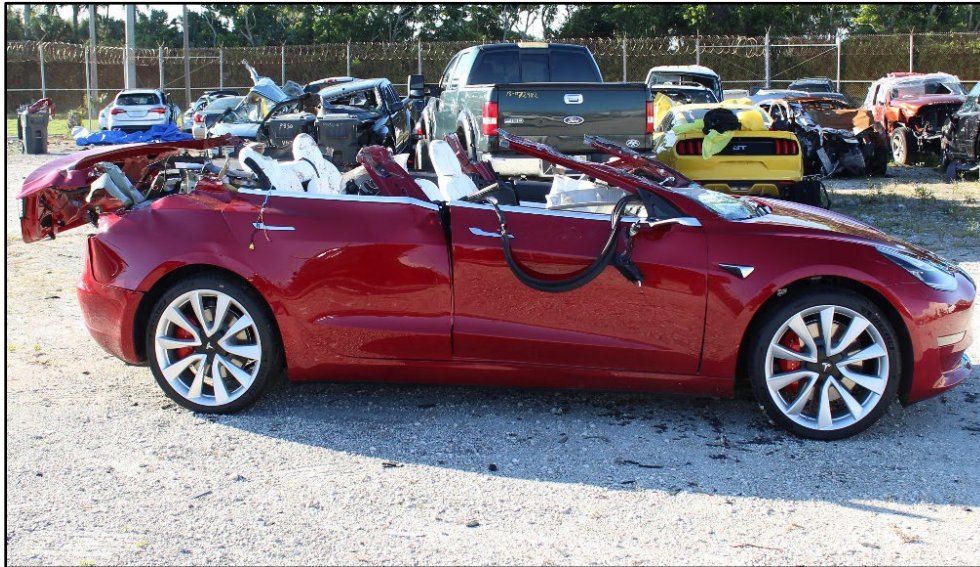
Figure 2. Tesla Model 3 with extensive roof damage photographed postcrash at tow yard.
